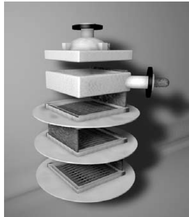
Tube side flow pattern, customized to achieve the required thermal and hydraulic performance.
