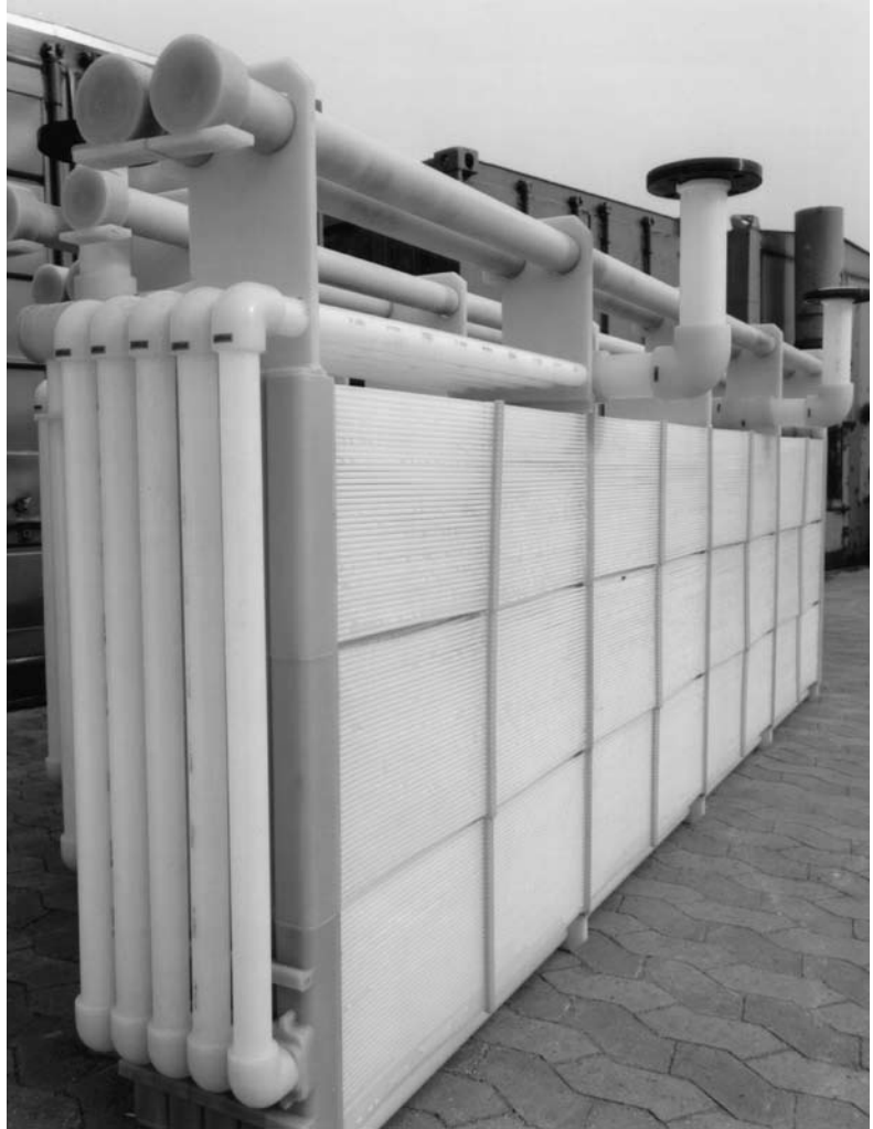
PVDF exchangers for cooling acid
