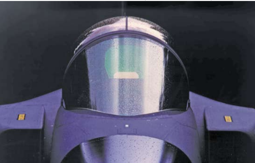
JAS 39 Gripen, windshield made from European GS 249 stretched
