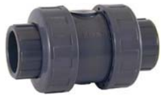
PVC TRUE UNION 1 O-rings: FPM (Viton®) 150 psi @ 73°F
