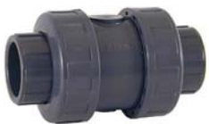
PVC TRUE UNION 1 O-rings: FPM (Viton®) 2 1/2" - 4" 150 psi @ 73°F
