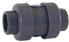
PVC TRUE UNION 1 O-rings: EPDM 2 1/2" - 4" 150 psi @ 73°F
