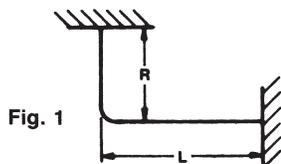
Normally, piping systems are designed with sufficient directional changes, which provide inherent flexibility, to compensate for expansion and contraction. To determine if adequate flexibility exists in leg (R) (see Fig. 1) to accommodate the expected expansion and contraction in the adjacent leg (L) use the following formula:
