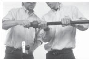
**CAUTION: Molten plastic material can cause severe burns. Avoid contact with the hot plastic and heat-tool. It is always a good idea to drape a thermal blanket over a hot heat-tool – Hand-held or bench-mount – when the installers must leave the work area. A – Caution Hot – sign, even crudely written on a cardboard box flap and posted on the workbench, is desirable when absent.**
