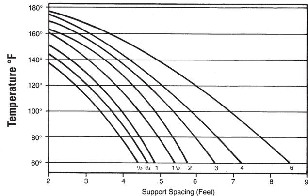
The above data is for uninsulated lines. For insulated lines, reduce spans to 70% of graph values. For spans of less than 2 feet, continuous support should be used.
