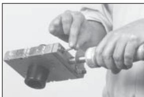
Give the Heating Anvils (heat face sets) a good spraying of silicone lubricant so that it will have a chance to "burn in" while they are heating up.
