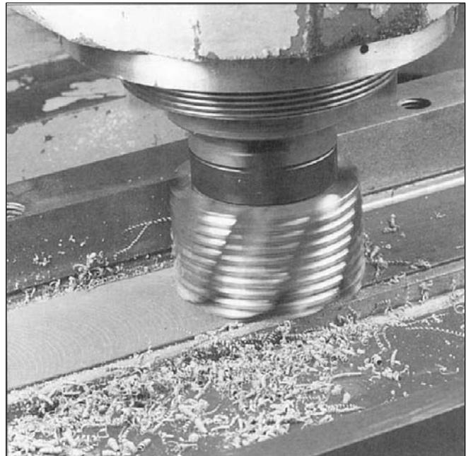
Figure 9 Precision Milling
