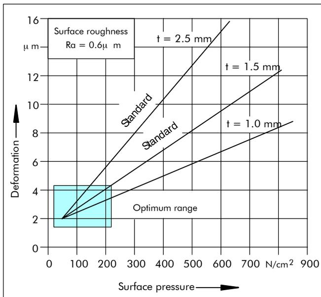
Figure 3 Deformation as a function of surface pressure and thickness  $t$  of the Turcite-B Slydway® material
