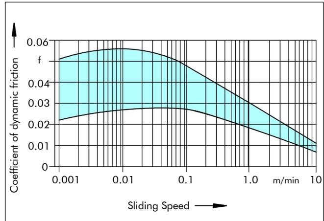
Figure 6 Range of the coefficient of dynamic friction (f) as a function of the sliding speed when using different lubricants
