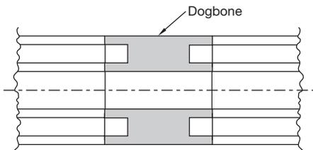
**Figure D-16. Locking inner and outer pipes**
