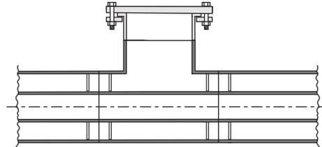
**Figure D-33. Access tee with flanged cover**
