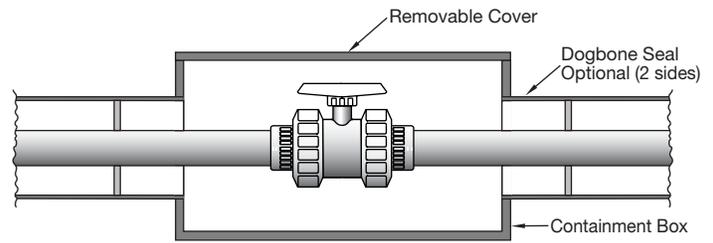
**Figure D-22. Double contained ball valve without stem extension: Poly-Flo system**
