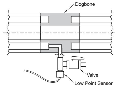
**Figure D-27. Connection with drain valve, Duo-Pro/Fluid-Lok systems**
