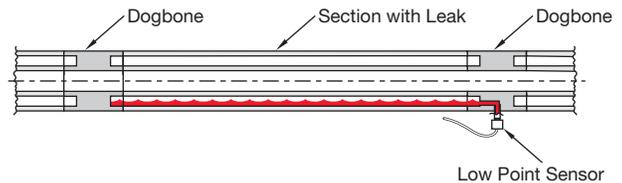
**Figure D-30. Leak detection compartments**
